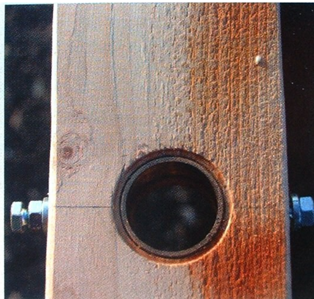
A section of metal piping, secured with furniture set screws, acts as a bushing in the rotator arm.
