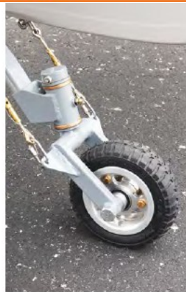
FIGURE 7: Tail wheel assembly fabricated by author in incorporating the suggested design features.
