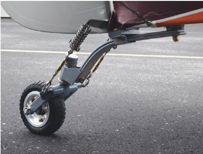
FIGURE 7: Tail wheel assembly fabricated by author in incorporating the suggested design features.
