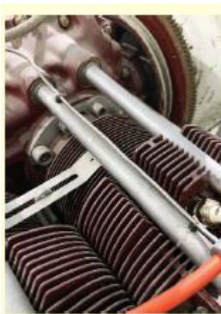
Improperly attached injector line
